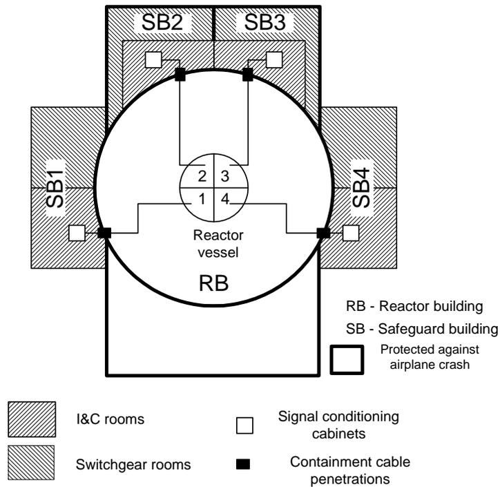
**G.5 FIG 6: INTERFACES AND RELATIONS BETWEEN REACTOR PRESSURE VESSEL
