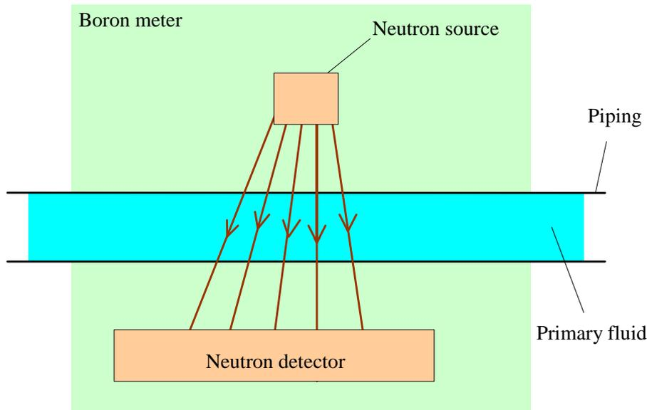
The role of the boron meters in the RCV[CVCS] is to provide on-line measurement of the boron concentration and to generate an alarm, or an automatic action, in case of exceedance of a limit which may be either fixed or calculated.
