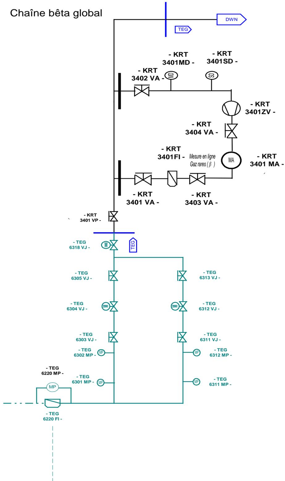
**Appendix 1.8: KRT [PRMS]/RPE [NVDS] Channel (Nuclear Auxiliary Building floor drain tank DP3)**
