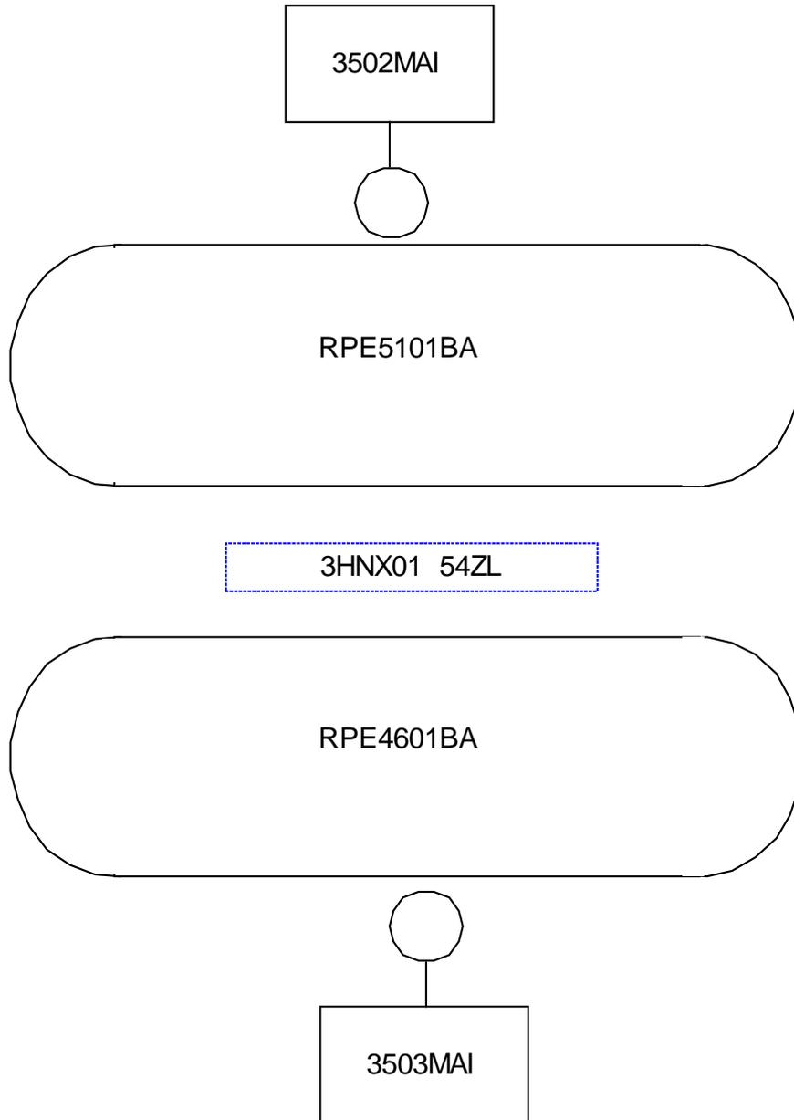
**Appendix 1.10: KRT [PRMS]/RPE [NVDS] Channels (Nuclear Auxiliary Building floor drain sump DP1)**
