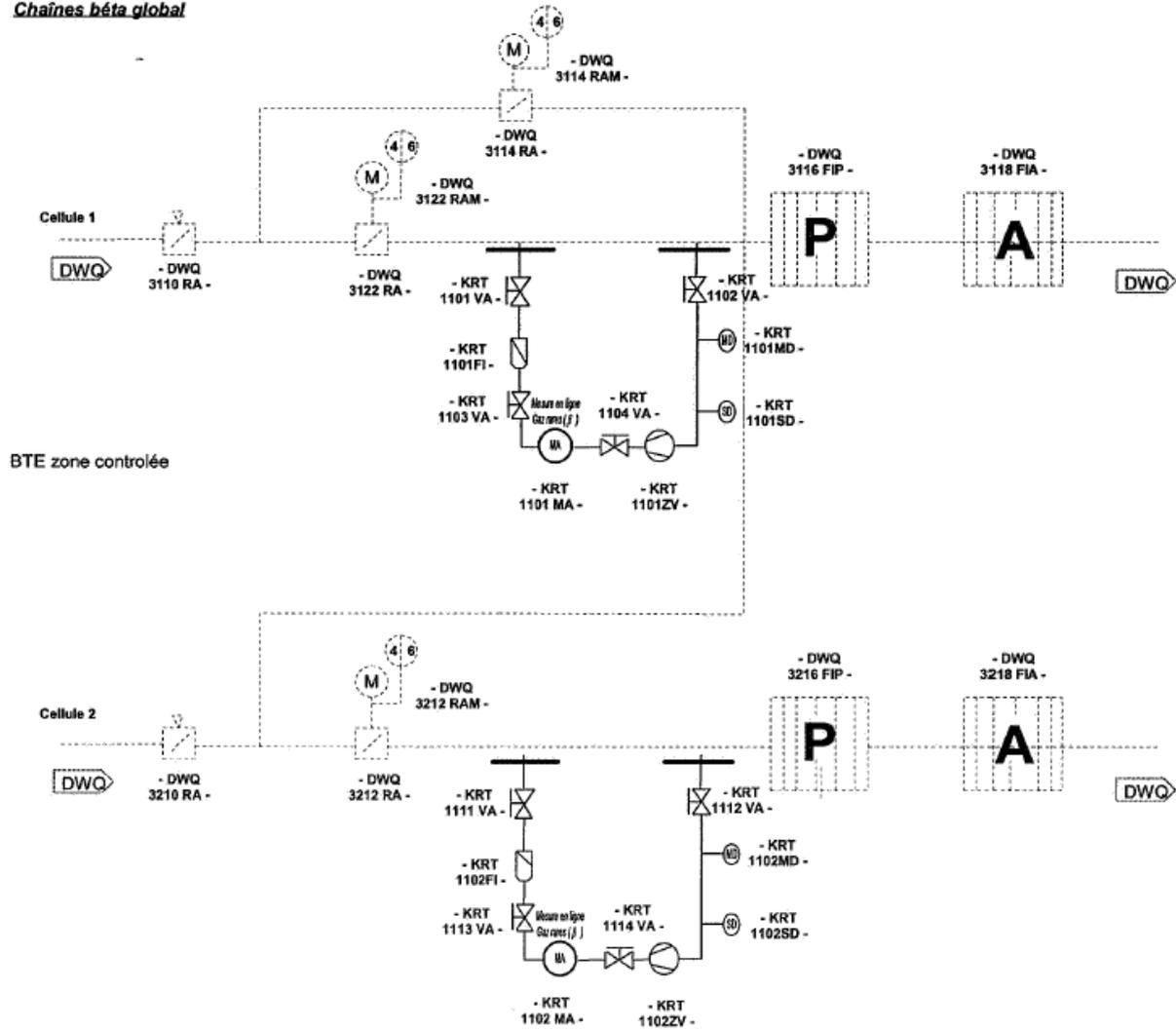
**Appendix 1.16: KRT [PRMS]/ Component Cooling Effluent Treatment system Channels**
