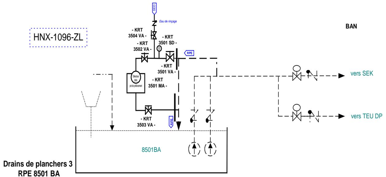
**Appendix 1.9: KRT [PRMS]/RPE [NVDS] Channels (Nuclear Auxiliary Building chemical drain tank DC and Nuclear Auxiliary Building residual drain tank DR)**
