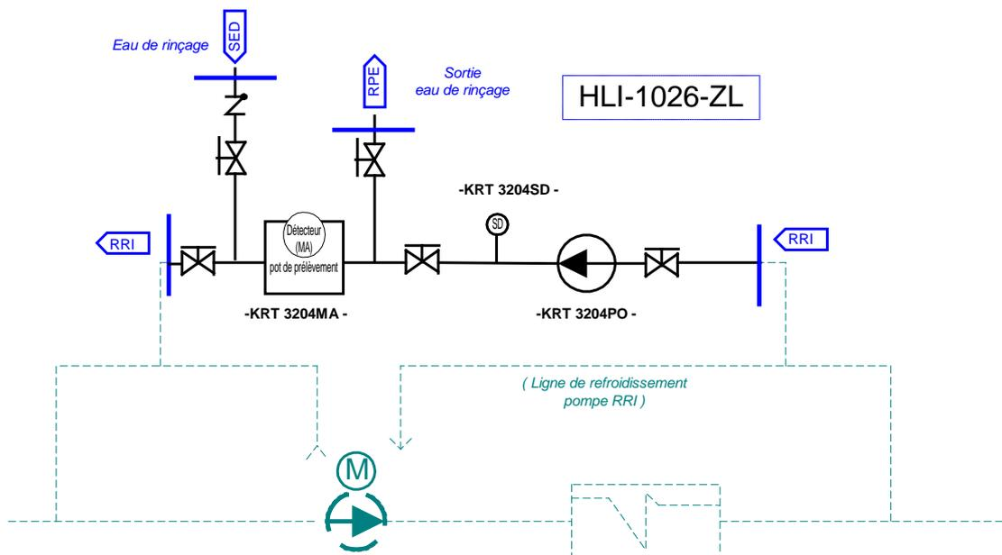
**Appendix 1.6: KRT [PRMS]/ Nuclear Auxiliary Building Ventilation System Channels
